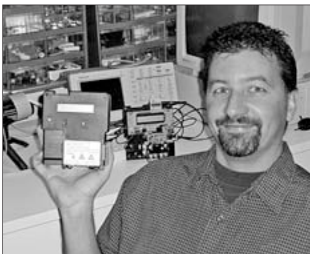
TIMELY DEVICE: The TightWatt, shown with inventor Stephen Allen, automatically adjusts pool timers seasonally.
